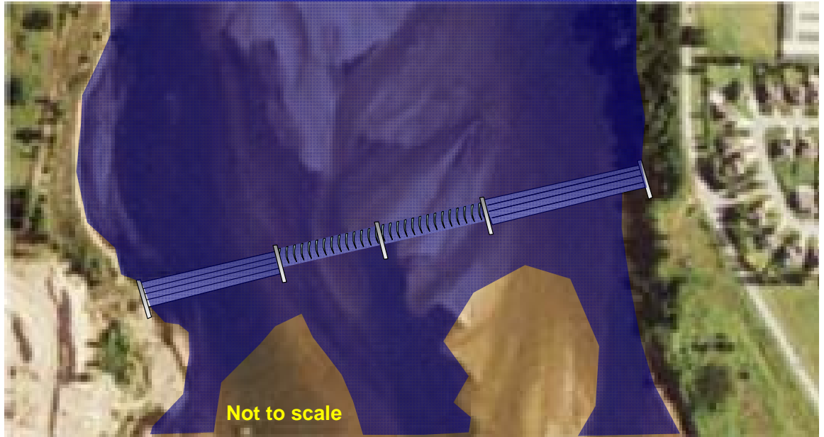
Figure 12. Visualization of Jenks Weir with Obermeyer Gate Sections and stepped Weir Sections Under Reregulation Flow Conditions
